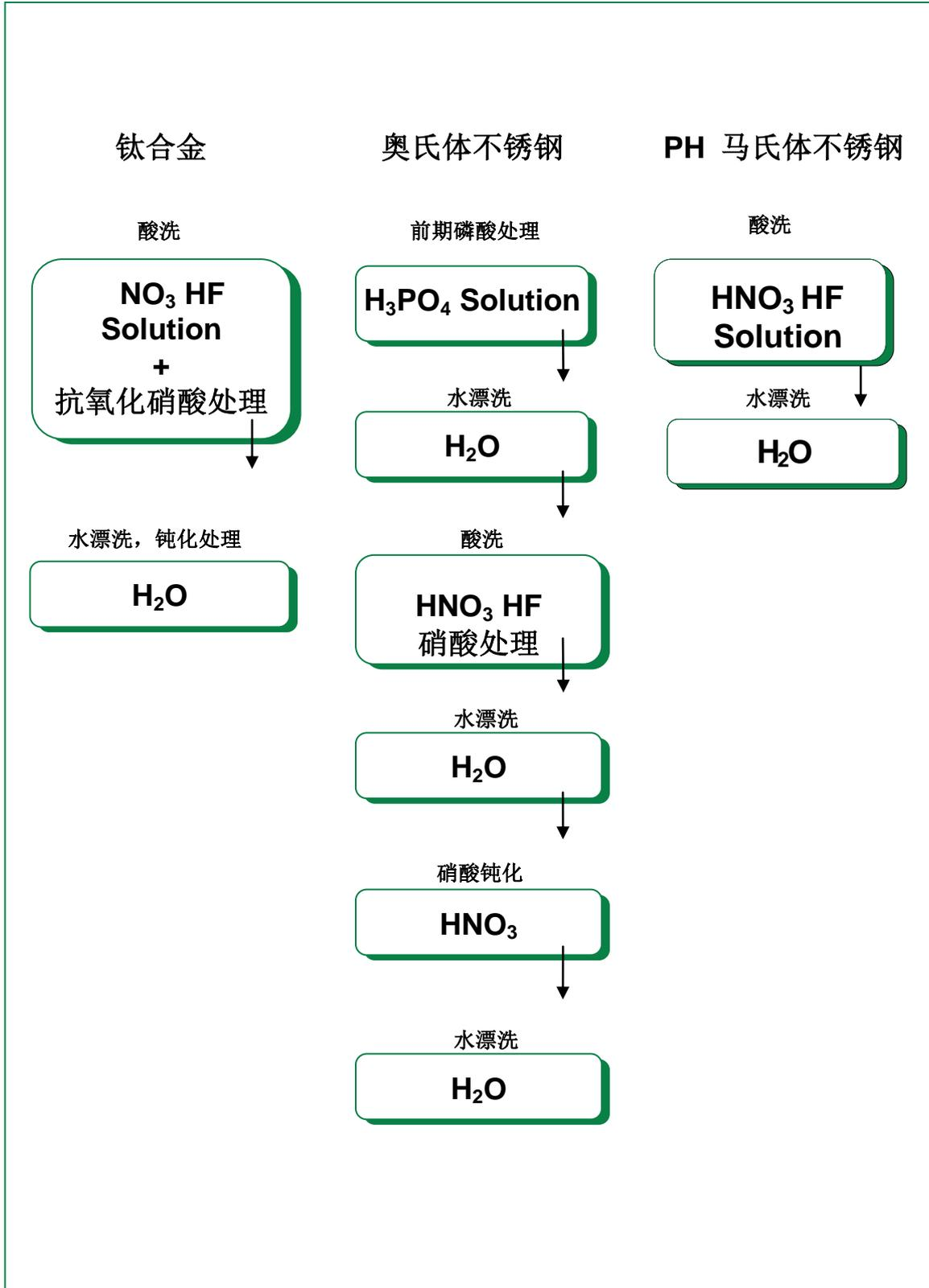
HOLE CLEANING OF CANNULATED BARS
